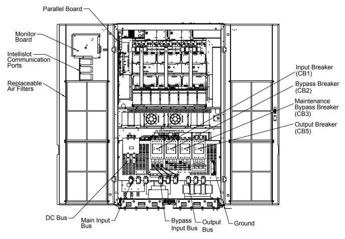
Figure 33 Liebert<sup>®</sup> NX<sup>™</sup> 160-200kVA main components—typical unit
